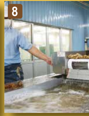
Factory workers check for leaves, grass, stones, etc., and break the Ukon into smaller pieces before they are cleaned in a small pool of jet water.
