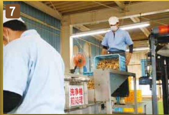
Harvested Ukon (turmeric) is pre-washed in Strong Kangen (pH11.0) water to loosen the soil.
