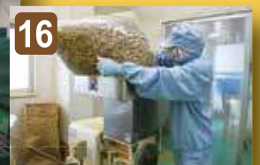
The factory is accommodated to process about 3.5 tons of Ukon in a day. By evening, this is made into about 500kg of dried Ukon.
