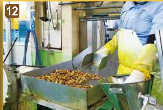
The Ukon is washed through a hot shower as it is loaded into the next room, where a worker scoops them into a slicing machine. The thin (1mm) sliced Ukon is gathered in a larger, wide container as it shoots out of the slicing machine.
