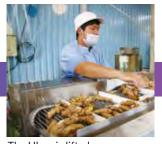
The Ukon is lifted on a conveyer belt where soil and any other impurities are sprayed off.
