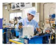
pH testing is also done during water flow testing on the completion line.
