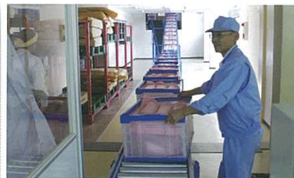
With the installation of the conveyor system, the transportation of parts has become smoother in the assembly section. 引入運輸帶之組合部門正運輸零件
