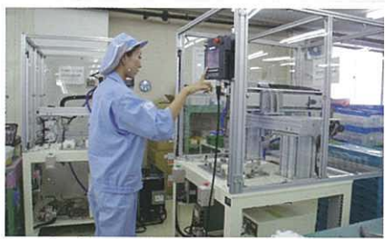
Productivity of the electrolytic chamber, the "heart of Leveluk", has doubled with the installation of two sophisticated screw-fastening machines in Department-3. 製造3課引入了2台最新端之電解槽裝配機“心臟部”之生產能力提升2倍
