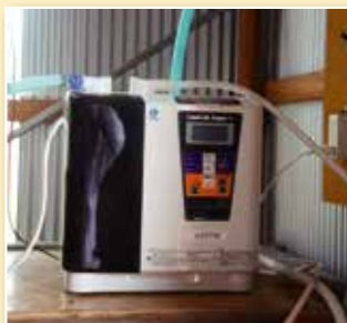
The Leveluk Super 501 unit that generates acidic electrolyzed water for disinfecting rice seeds Leveluk Super501產生的酸性電解水用於消毒稻米種子
