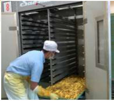
The Ukon trays are slid into a heat-dryer for about 7 hours in 72°C (161.6F °).
