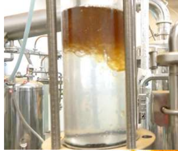
A higher concentration of turmeric is slowly extracted through another 3-hour process for use in the UkonΣ and Ukon Soap.
